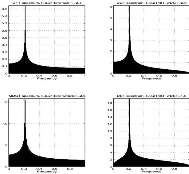
Fig. 3 Examples of spectra of sinusoidal signals with random frequency in the range [54.5-55.5] in the window of 512 samples (no window function). For the display purpose, spectral magnitudes are risen to the power 0.3. wDFT, wDCT, wMDCT and wDST show peak width on the energy level 0.9.
