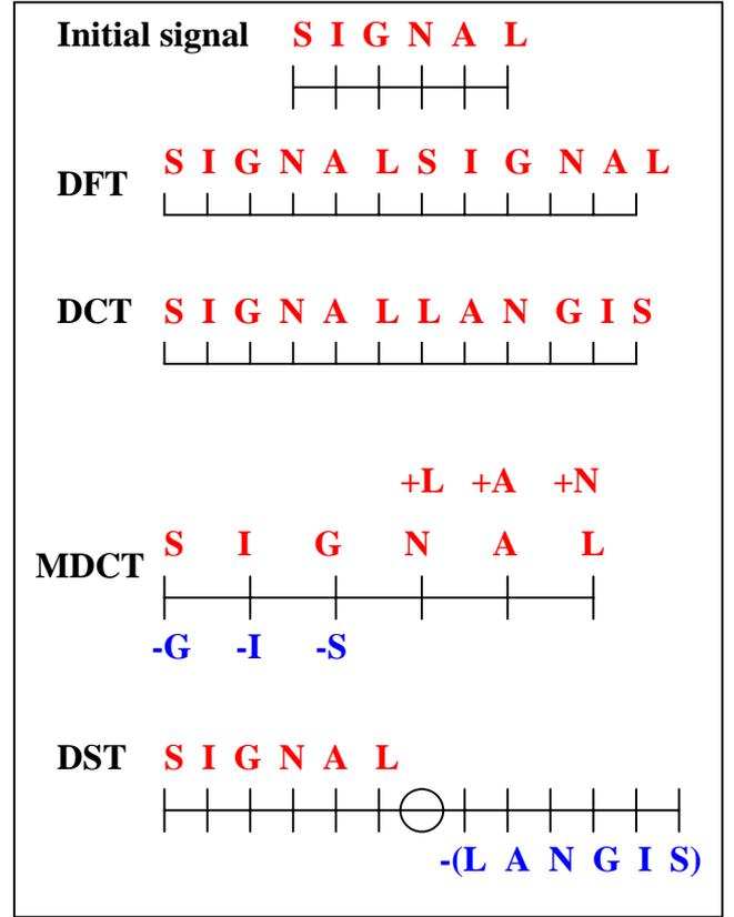
Fig. 1 Signal and its corresponding representations for DFT, DCT, MDCT and DST
