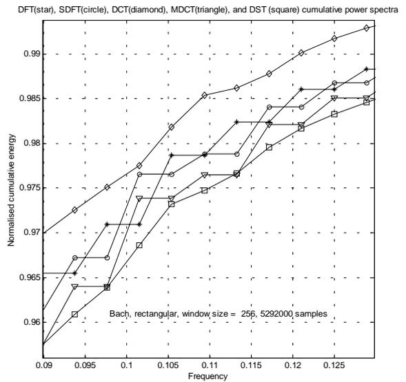
Fig. 4. An example of comparison of convergence of spectra in different bases of a piece of 5292000 samples of Bach music for window size of 256 samples. For each frequency, the data show fraction of total signal energy that is contained in the bandwidth bounded by this frequency
