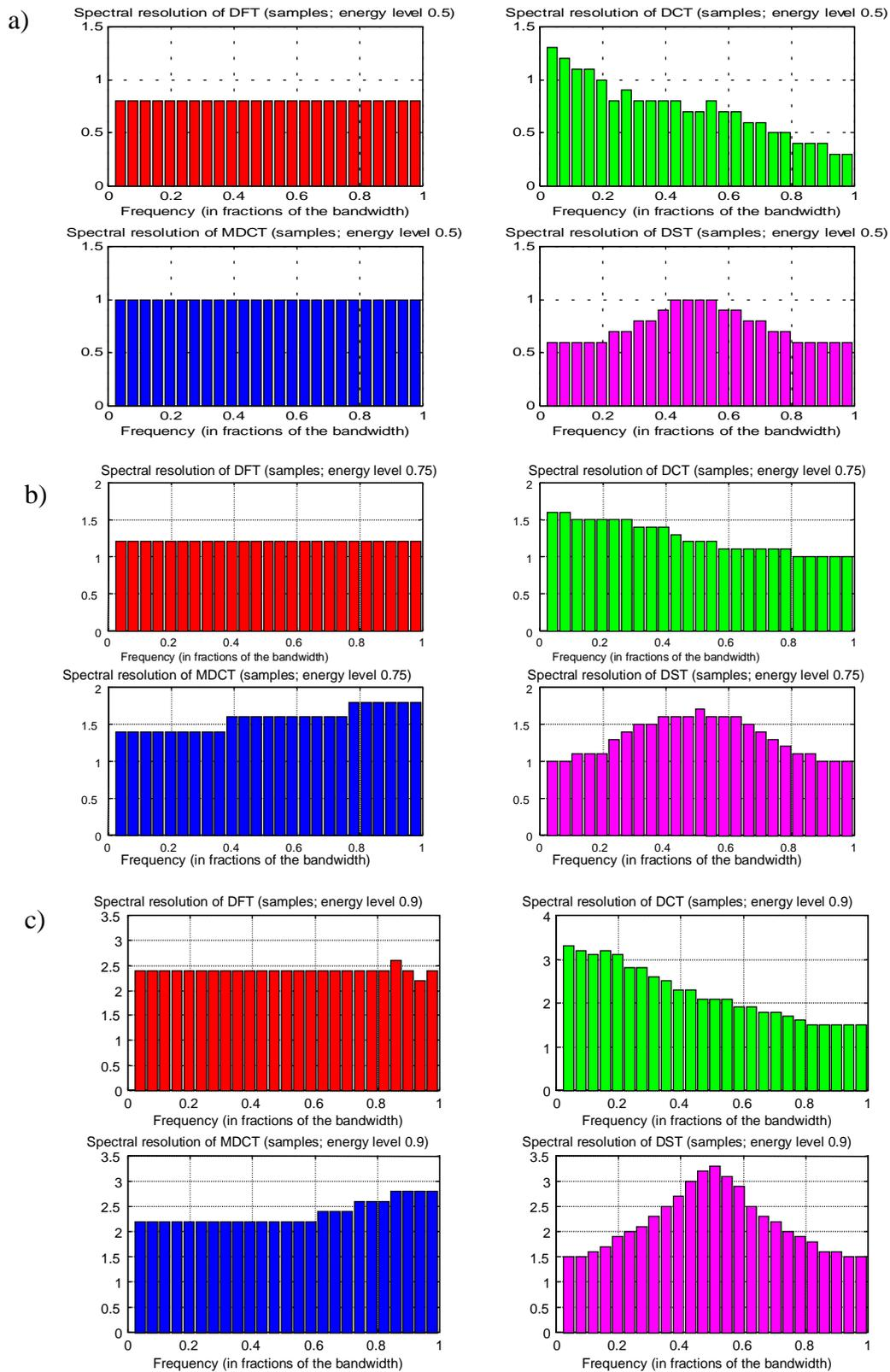
Fig. 2 4 Comparison of spectral resolution (width of signal spectrum) of DFT, DCT, MDCT and DST for sinusoidal signals of 512 samples as a function of signal frequency for different energy levels: a) 0.5; b) 0.75; c) 0.9.
