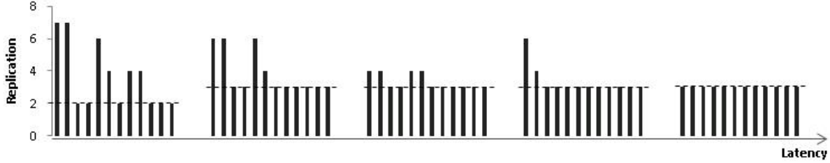
Figure 5: Replication factors for instances of filter CombineDFT in FFT. The dotted line separates the replication required to achieve the maximum throughput for a specific design point from the additional replication introduced to decrease latency.
