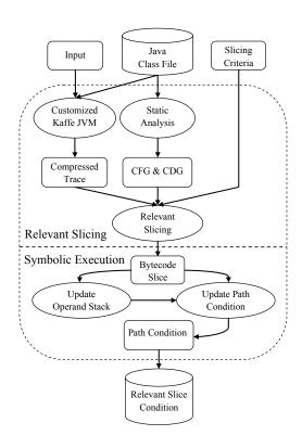
Figure 6.9: Architecture of relevant-slice condition computation
