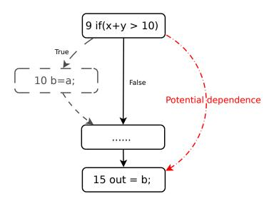
Figure 6.3: Example of potential dependence. The solid arrows denote the execution path. According to Definition 6.15, (i) the variable *b* is not defined between line 9 and line 15 but there exists a path (though line 10) along which *b* is defined, and (ii) evaluating the branch at line 9 differently may cause the path through line 10 to be executed. Therefore, line 15 is potentially dependent on line 9.
