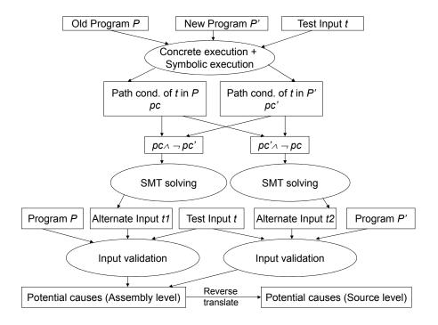
Figure 5.3: Architecture of our DARWIN toolkit. It takes an old program P, a new program P' and a test input t which passes in P but fails in P'. The output is a report explaining the behavior of test t. The entire flow is automated.
