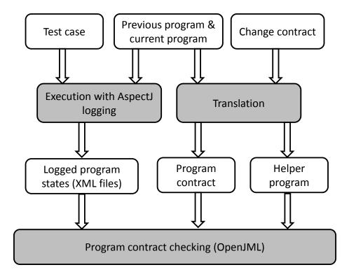
Figure 7.7: The architecture of change contract runtime checker
