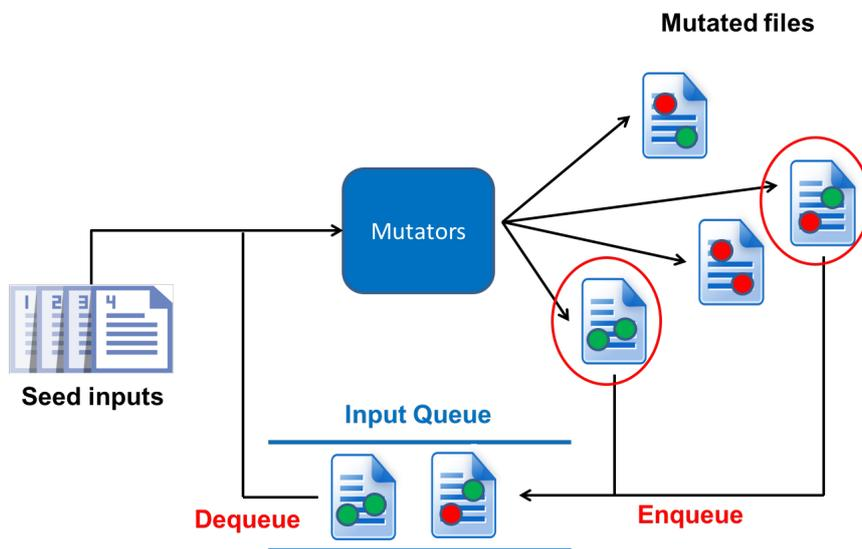
Figure 2-6: Architecture of AFL as a File Fuzzer
