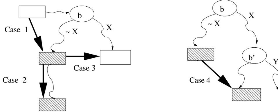
**Figure 5.2:** Additional edges in the Cache Conflict Graph due to Speculative Execution. The l-blocks are shown as rectangular boxes, and the ml-blocks among them are shaded.
