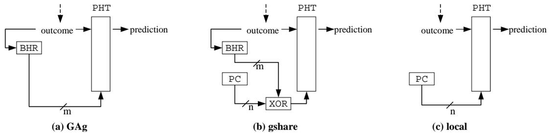
**Figure 2.3:** Illustration of Branch Prediction Schemes. The branch prediction table is shown as PHT, denoting Pattern History Table.
