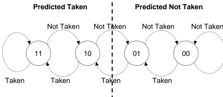
**Figure 2.4:** Two-bit Saturating Counter Predictor
