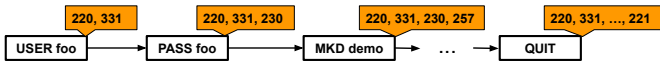
Fig. 3. An annotated FTP message sequence processed for mutational fuzzing (from the sniffer trace in Listing Listing 1)
