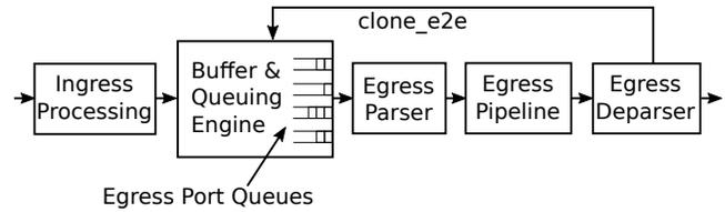
Figure 1: General architecture of a programmable switching ASIC [10]
