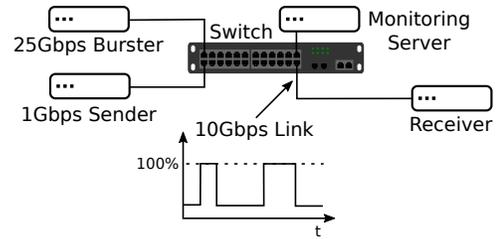
**Figure 4: Testbed setup**
