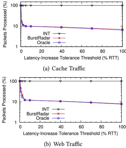
**Figure 5: Fraction of total number of packets processed for different latency-increase thresholds**
