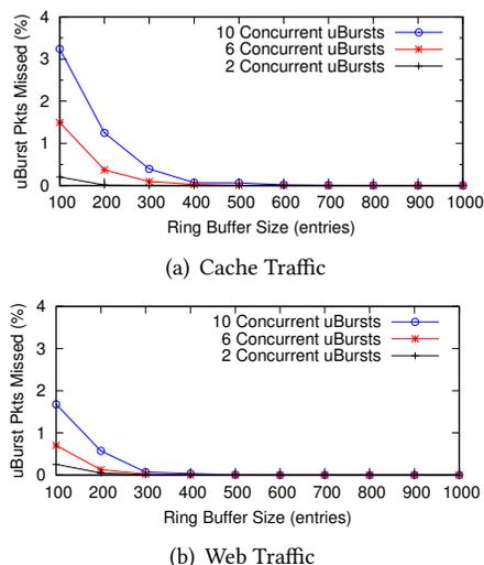
**Figure 7: Fraction of microburst packets missed with concurrent microbursts for different ring buffer size**
