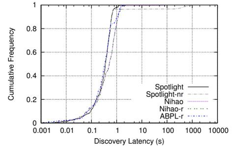
Fig. 19: Discovery Latency CDF for 1 ms slot size at 1% duty cycle.
