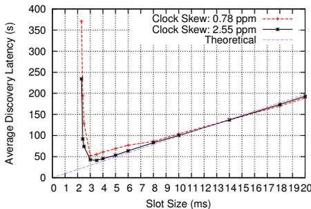
Fig. 2: Average pairwise discovery latency for two pairs of nodes.
