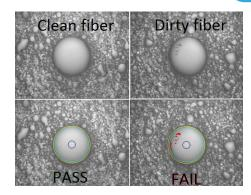
Fiber Contamination Airborne dust particles
