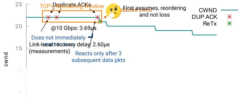
We can retransmit a lost packet out-of-order within TCP's reordering window:
