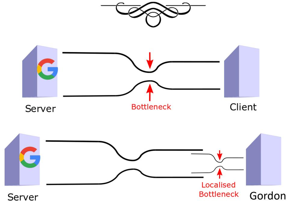
Most network dynamics, like change in bottleneck bandwidth and packet losses happen at the connection bottleneck. Localizing the bottleneck allows us to have better control over the connection.
