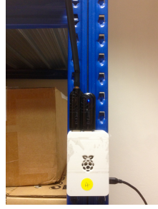
(b) Raspberry pi monitor deployed with two dongles
