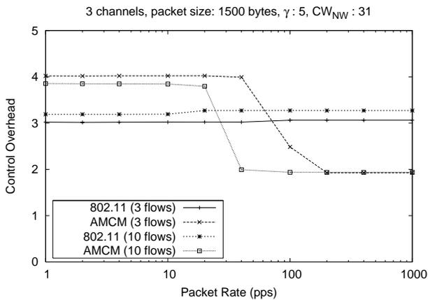
Figure 7. WLAN: Comparison of control overhead against IEEE802.11
