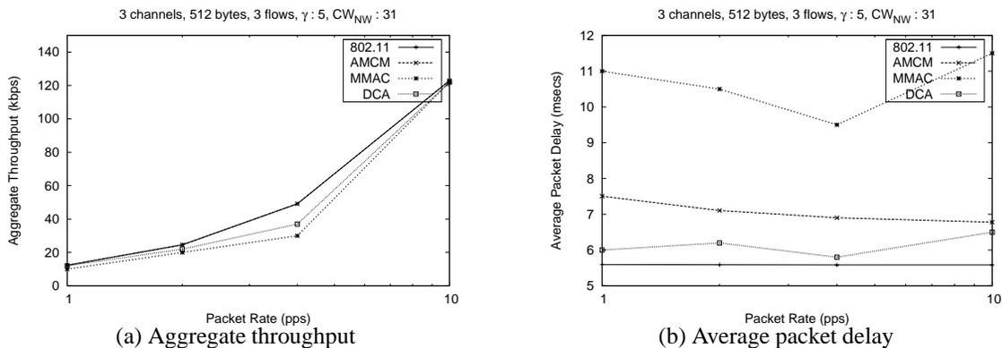
Figure 6. WLAN: Performance impact under low load
