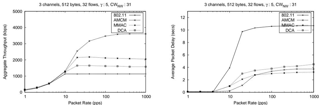
Figure 5. WLAN: Impact of traffic load on aggregate throughput and delay
