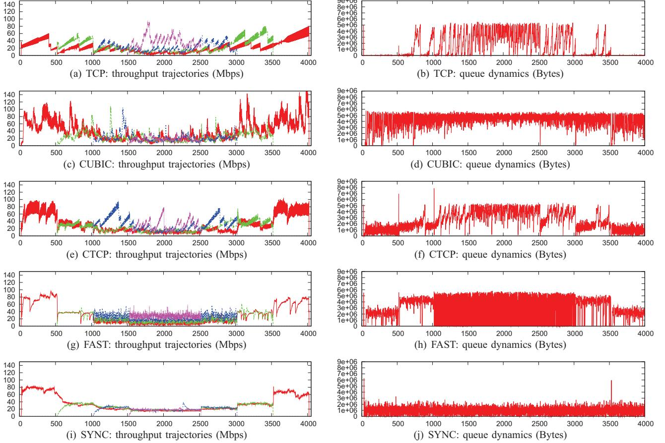
Fig. 9. Dynamic Scenario: throughput trajectories of flow 0, 10, 20, 30 (left) and queue dynamics of the bottleneck link (right)
