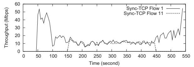
Fig. 16. Throughput Trajectory of Two Sync-TCP Flows
