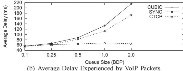
Fig. 14. Effects of Different Buffer Sizes (Testbed Evaluation)
