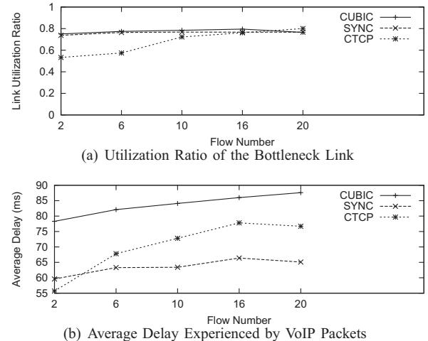
Fig. 13. Scalability with Flow Number (Testbed Evaluation)
