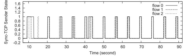
Fig. 12. Synchronization of Congestion Detection through Queue Delay
