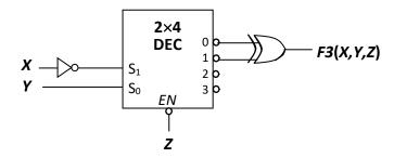
Answer:  $F3(X, Y, Z) = (Z + X' + Y)' \cdot (Z + X' + Y') + (Z + X' + Y') \cdot (Z + X' + Y')' = Z' \cdot X \cdot Y' + Z' \cdot X \cdot Y = X \cdot Y' \cdot Z' + X \cdot Y \cdot Z' = \Sigma m(\mathbf{4}, \mathbf{6}).$
