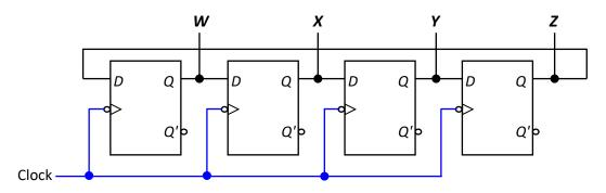
Suppose the circuit is initialised with the value *WXYZ* = 0101, how many unique states does the circuit cycle through?
