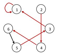
(b) A circuit is **self-correcting** if for some reason the circuit enters into any unused (invalid) state, it is able to transit to a valid state after a finite number of transitions. Is this circuit self-correcting? Explain.
