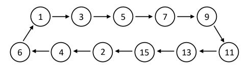
The states are represented by 4-bit values *ABCD*. Implement the sequential circuit using a *D* flip-flop for *A*, *T* flip-flops for *B* and *C*, and a *JK* flip-flop for *D*.
