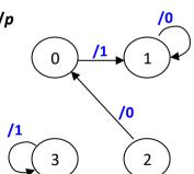
(b) After 3 clock cycles, the circuit is in state 1, and it generated 100 as output.
