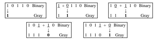
Given a half-adder as shown on the right where X and Y are its inputs and C (carry) and S (sum) its outputs, implement a 5-bit binary to Gray code converter to convert the binary value ABCDE to its equivalent Gray code PQRST by using the fewest number of half-adders without any additional logic gates.
