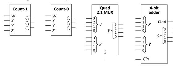
Given the above 4 components, you are to employ block-level design to design the converter, without using any additional logic gate or other devices. You may observe that if A = 1, then the output FGH is simply the number of 1s in the input ABCD. You are to make your own observation for the case when A = 0.
