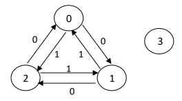
A circuit is **self-correcting** if for some reason the circuit enters into any unused (invalid) state, it is able to transit to a valid state after a finite number of transitions. Is your circuit self-correcting, and why?
