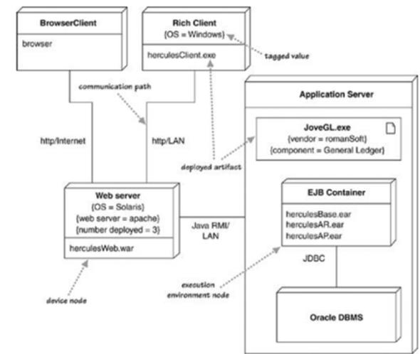
Deployment diagrams show a system's physical layout, revealing which pieces of software run on what pieces of hardware.
