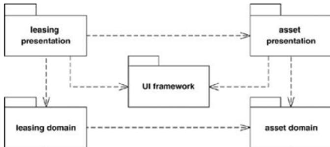
A package diagram shows packages and their dependencies. A package is a grouping construct for grouping UML elements (classes, use cases, etc.).
