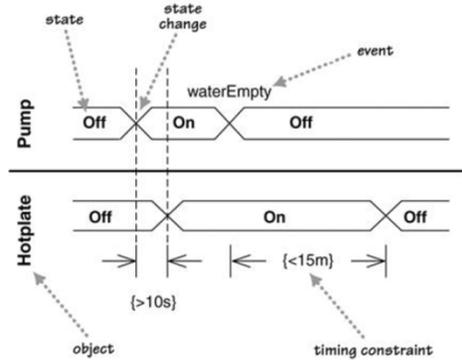
Timing diagrams focus is on timing constraints.
