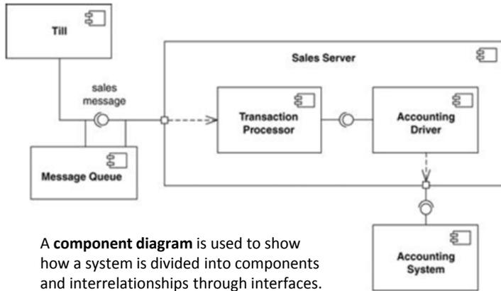
A component diagram is used to show how a system is divided into components and interrelationships through interfaces.
