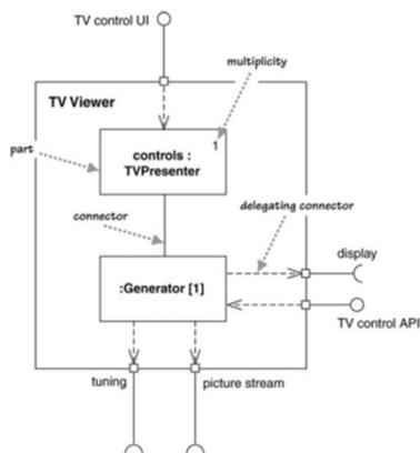
A composite structure diagram hierarchically decomposes a class into its internal structure.
