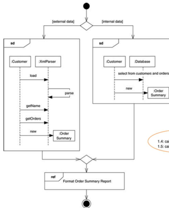
Interaction overview diagrams are a combination of activity diagrams and sequence diagrams.
