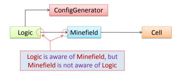
At the level of program code, navigability implies how objects are referenced. In the example above, a Logic object holds a reference to a ConfigGenerator object, but not the other way around. Navigability can be *unidirectional* or *bidirectional*. For convenience, a line without arrow heads can be used to indicate a bidirectional link. However, if none of the associations in a class diagram has navigability arrows, it usually means that navigability is "unspecified".
