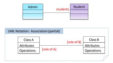
Note that an association link in a class diagram denotes a permanent or semi-permanent structural link between objects of two classes. Temporary contacts between objects (e.g. ClassA uses a constant defined in ClassB) are not shown as associations. Such temporary contacts are shown as *dependencies* instead (denoted as a dashed arrows).
