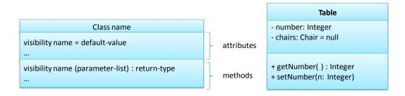
The above illustrates the basic notations of a class diagram. In particular, attributes represent the data of the class, as opposed to methods that represent the operation (or behavior).
