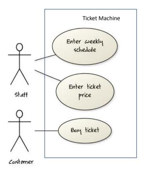
Note that most of the details in the description are better given as part of the use case description rather than as low-level use cases in the diagram.
