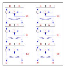
Each of the 16 stages (rounds) of DES uses a Feistel structure which encrypts a 64 bit value into another 64 bit value using a 48 bit key derived from the original 56 bit key.
