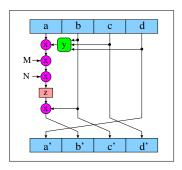
One round of 64, performed for each 512 bits of the input.  $\langle a, b, c, d \rangle$  are four 32-bit registers. At the end they contain the 128 bit value of the checksum.
