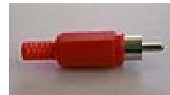
Mono-TS Jack and RCA are unbalanced
