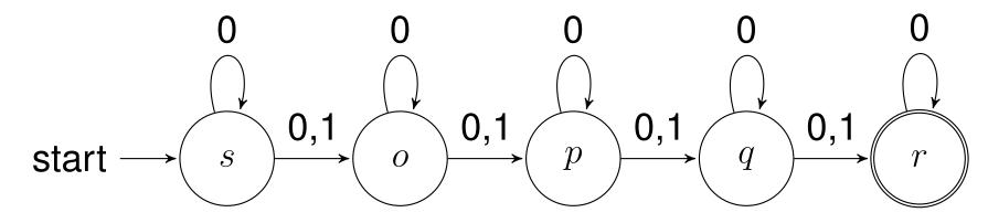
Input 00111: Accepting runs s(0) s(0) o(1) p(1) q(1) r and s(0) o(0) o(1) p(1) q(1) r; the rejecting run s(0) s(0) s(1) o(1) p(1) q is not relevant. Input 11111: No accepting run; only possible run s(1) o(1) p(1) q(1) r(1) ... gets stuck. Input 000: No run reaches accepting state r in time, s(0) o(0) p(0) q is fastest run and falls short of final state. Quiz: How many runs for 1001001 are accepting?
