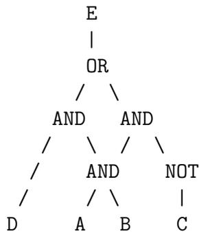
The number of layers is called the depth of the circuit. Here there are three layers of gates, each causing one delay. If one does not have a multiple input for the above
