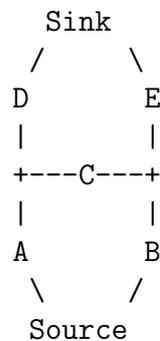
The first circuit is for  $(A \wedge B) \vee (\neg A \wedge \neg B)$ ; the second for  $(A \wedge D) \vee (A \wedge C \wedge E) \vee (B \wedge C \wedge D) \vee (B \wedge E)$ . The surprising usage of input  $C$  is that it might allow flows in either direction.
