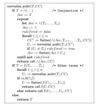
Fig. 1. Basic ACDTR normalisation algorithm.
