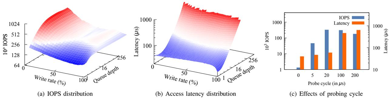
Fig. 3. The effects of queue depth, write rate and probe cycle to the performance of NVM device.
