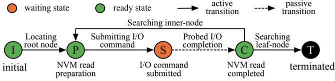
Fig. 5. The state transition graph for the point search operation.
