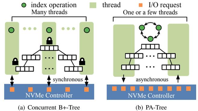
Fig. 1. Comparison between the synchronous execution paradigm (left) and pull-mode asynchronous execution paradigm (right) under NVMe interface.
