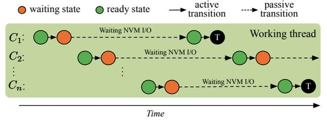
Fig. 6. The demonstration of asynchronous execution of  $n$  operations.
