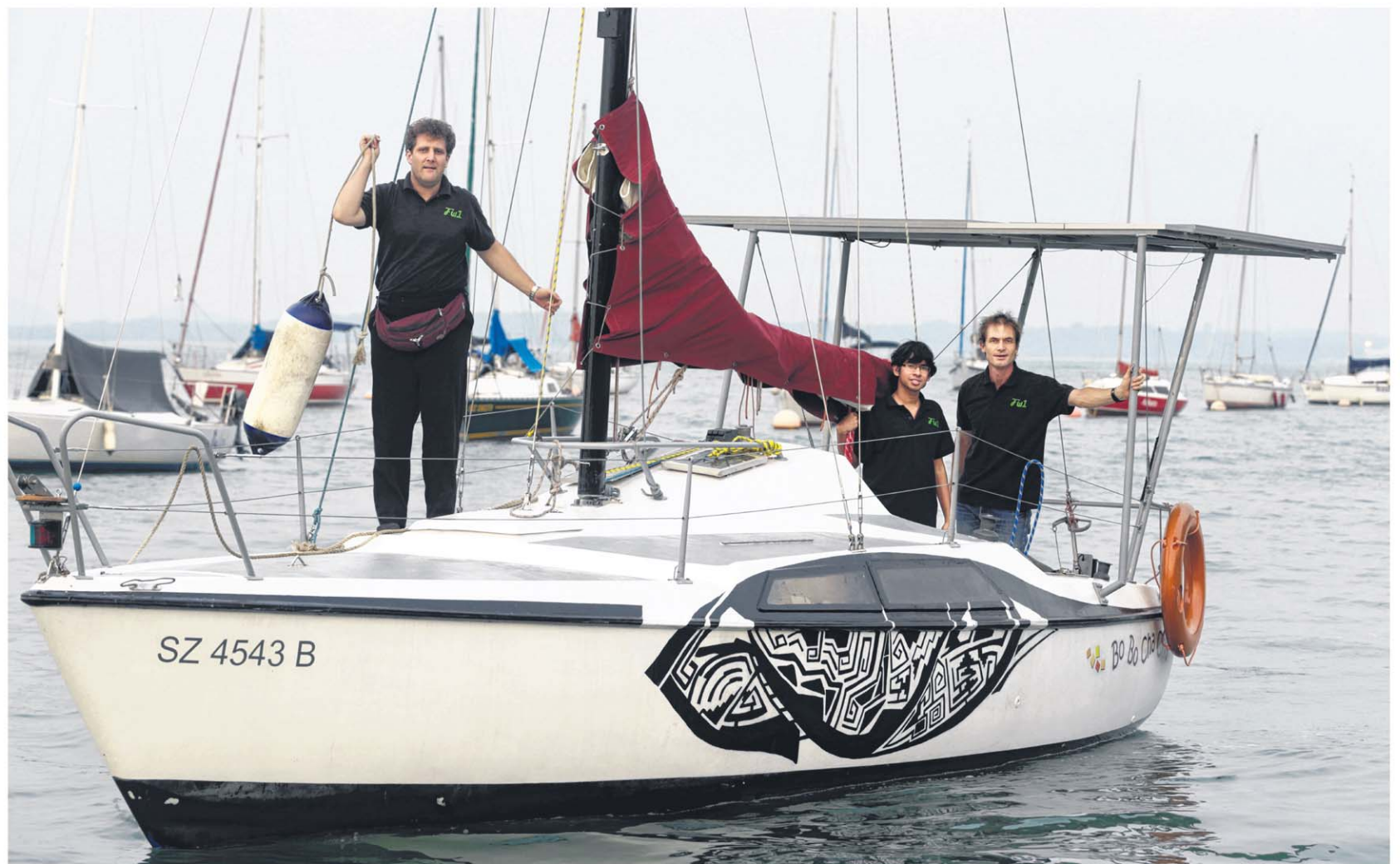
(From left) Dr Joerg Weigl, Mr Anand Sundaram and Associate Professor Martin Henz on board the Bo Bo Cha Cha at Changi Sailing Club. Without using its sail, the zero-carbon boat can travel for five hours non-stop, with a full speed of 5 knots, or about 9kmh. ST PHOTO: NEO XIAOBIN
