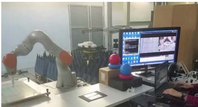
Figure 2. Structure of physical robot drawing system.
