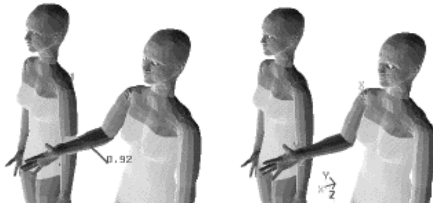
Figure 8. Multi-actor collision detection and correction with inverse kinematics, the guiding frame displayed in the right figure is derived from the response vector.
