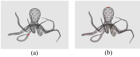
Figure 2. Automatically (a) and interactively (b) selected root vertex: (a) usually located at the tip of a longest branch and (b) at polar extremity
