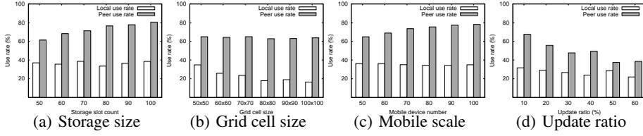
Fig. 10. Storage Use Rate in MANET Simulation
