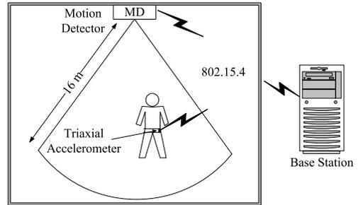
Fig. 1. Wireless system of body-worn and static sensors
