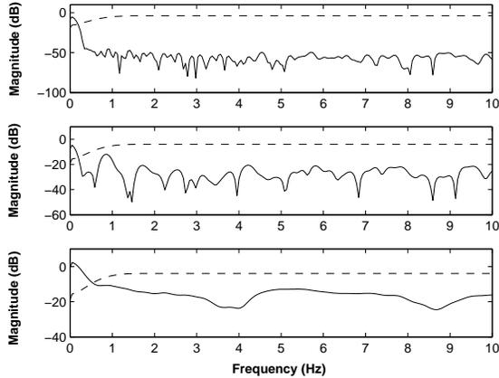
Fig. 2. Magnitude spectrum of acceleration data corresponding to various activities. The solid line represents the magnitude spectrum of acceleration in the horizontal direction and the dashed line represents the magnitude spectrum of the high-pass filter used to obtain the dynamic acceleration. The top plot corresponds to standing, the middle plot walking and the bottom plot falling.
