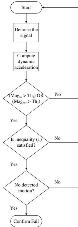
Fig. 4. Detection algorithm flowchart
