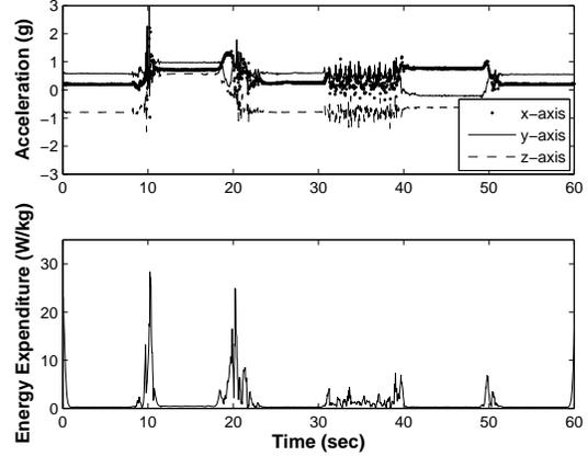
Fig. 3. Using triaxial acceleration data to estimate energy expended in performing various activities. The top plot shows the acceleration data corresponding to the following sequence of activities: standing, falling, standing, walking, sitting and standing. The bottom-plot shows the estimated energy expended in performing these activities.
