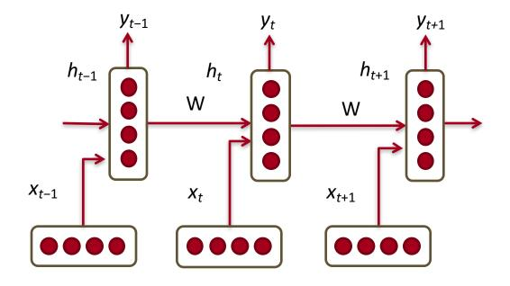
Given list of word vectors:  $x_1, \ldots, x_{t-1}, x_t, x_{t+1}, \ldots, x_T$ At a single time step:  $h_t = \sigma \left( W^{(hh)}h_{t-1} + W^{(hx)}x_{[t]} \right)$  $\hat{y}_t = \operatorname{softmax} \left( W^{(S)}h_t \right)$
