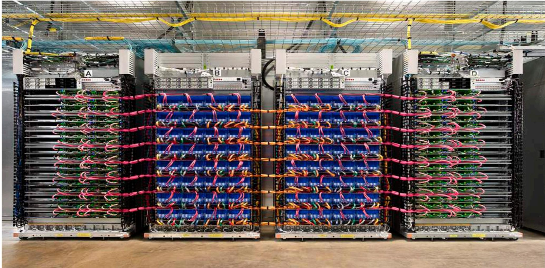
A “TPU pod” built with 64 second-generation TPUs delivers up to 11.5 petaflops of machine learning acceleration.
