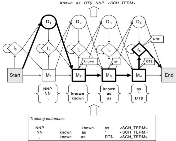
**Figure 3. Generating a test instance with gaps using the PHMM. The optimal path is in bold, and words or tags emitted are shown in callouts.**
