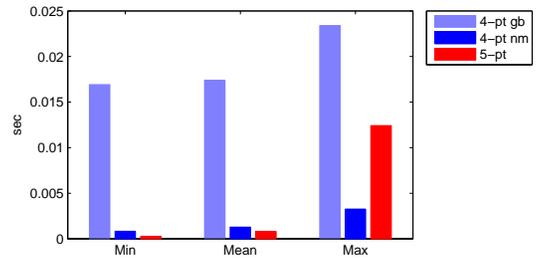
Fig. 1. Computation time for the minimal case for the various relative pose estimation algorithms. 4-pt gb stands for the closed-form Groebner basis solver. 4-pt nm stands for the numerical solver using gradient descent.
