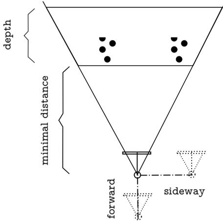
Fig. 2. Experiment settings for simulation data. The two dashed cameras mark the locations to which the camera moves with forward and sideways motion respectively.
