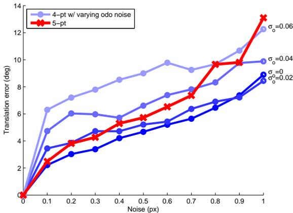
Fig. 4. Translation error in degrees against noise standard deviation in pixels. The standard deviation  $\sigma_\theta$  of the relative rotation angle measurement noise ranges between 0 and 0.06. 50 points are used to execute a RANSAC scheme for each test.
