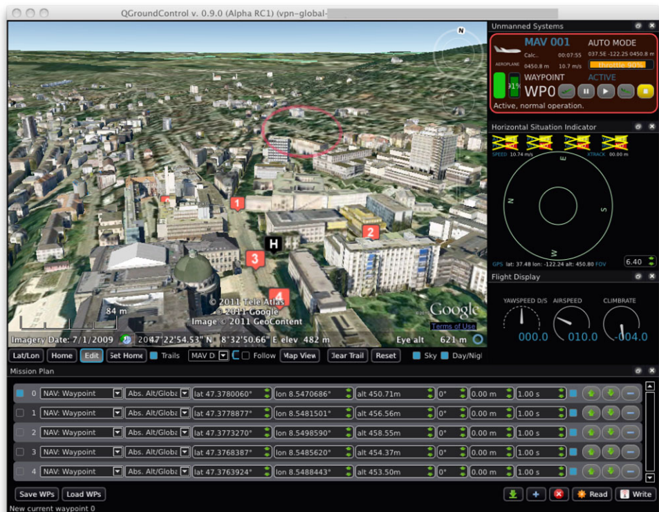
Fig. 10 QGroundControl displaying the current waypoints and trajectory of the system
