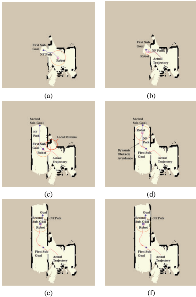
Fig. 12. Snapshots of the trajectories and acquired maps of the Nomad XR4000 mobile robot during the implementation of the integrated algorithm. The blue lines represent the navigation function (NF) path from the robot to the respective sub-goals and red lines represent the actual trajectories taken by the robot.
