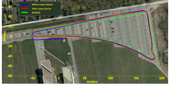
Figure 9. Trajectories before and after pose-graph loop-closure compared with GPS/INS ground truth.
