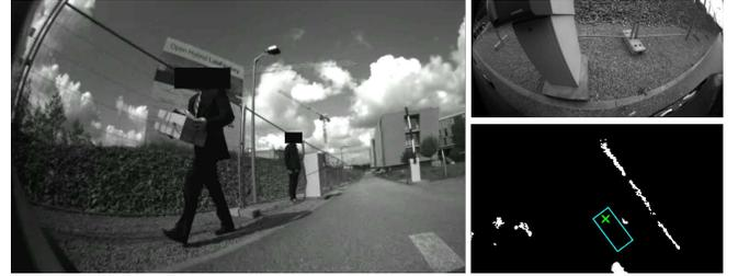
Fig. 13: Difficult situations for the local motion planner. Pedestrians moving in close proximity to the car (left) and passing through narrow gates (right).
