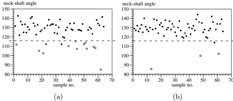
**Fig. 3.** Measured neck-shaft angles of training images. (a) Left femurs. (b) Right femurs. Dots: healthy femurs, squares: fractured femurs, dashed line: decision threshold.
