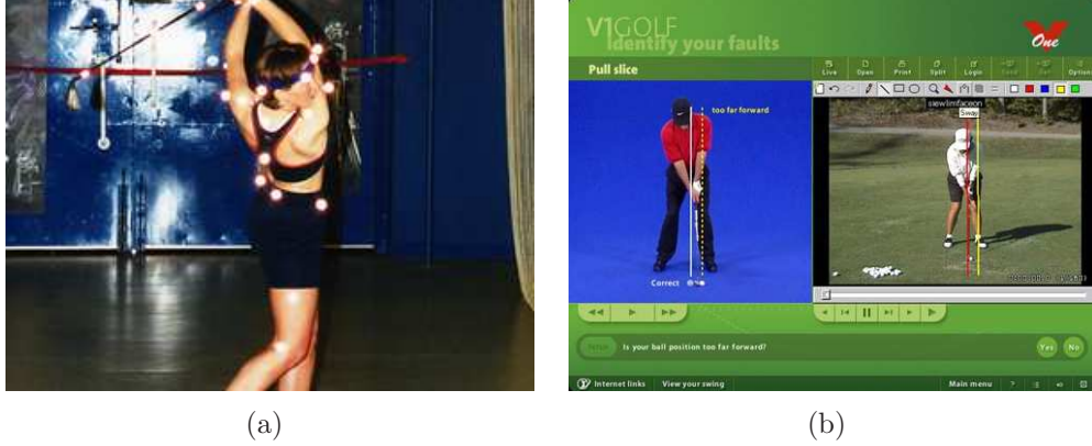
Figure 1.1: Commercial systems for sports motion analysis. (a) Vicon 3D motion capture system captures a performer’s golf swing using reflective markers attached to the human body (from http://www.vicon.com/applications/sports.html ). (b) V1 Golf Software requires manual comparison of the performer’s postures with those of an expert (from http://www.ifrontiers.com/consumer/default.asp ).
