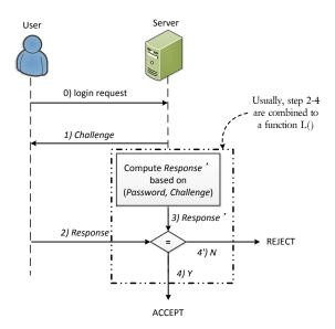
Figure 1. Typical steps in Response-Computable Authentication (RCA).
