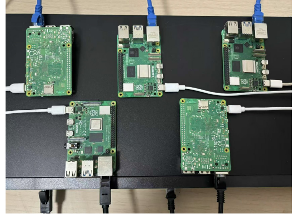
Fig. 3: Our 5-device example experimental prototype utilizes a switch and Raspberry Pi 4B devices, with one dedicated to the fusion model and the other four allocated to sub-models.
