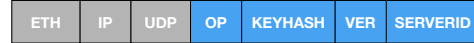
Figure 2: Pegasus packet format. The Pegasus application-layer header is embedded in the UDP payload. OP is the request or reply type. KEYHASH contains the hash value of the key. VER is an object version number. SERVERID contains a unique server identifier.
