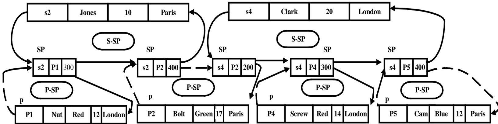
Fig. 16. A suppliers-and-parts database instance
