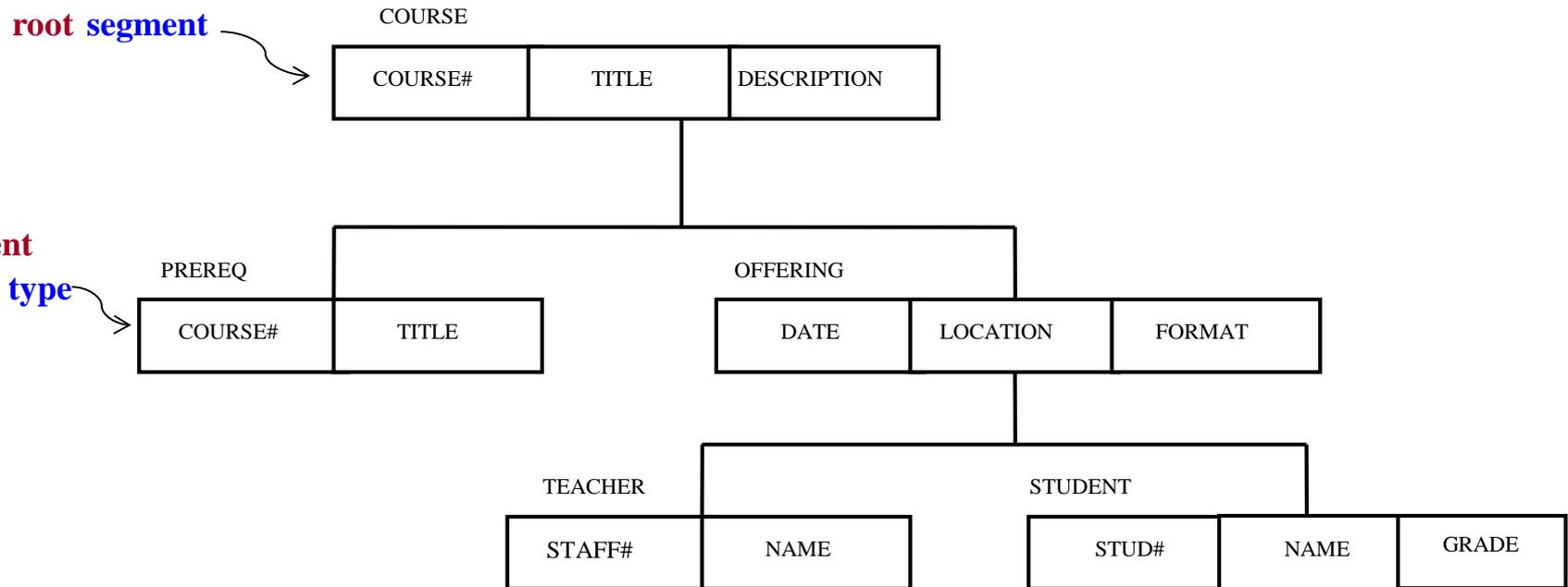
Fig. 1. PDBR (physical database record) type for the education database (schema)
