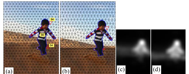
Figure 4: (a) Input image with triangle mesh. Yellow rectangles show the average luminance ( $L^*$ ) values in the subject and the red triangles. (b) Output image. Triangles have been expanded and compressed accordingly. (c & d) Saliency maps from input and output images respectively.
