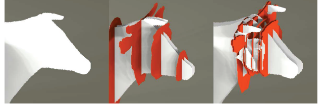
Fig. 13. Cow sliceforms using different values of \tau_A and number of dominant slicing directions: (left) 0.05 and 1, (middle) 0.05 and 2, and (right) 0.015 and 1.
